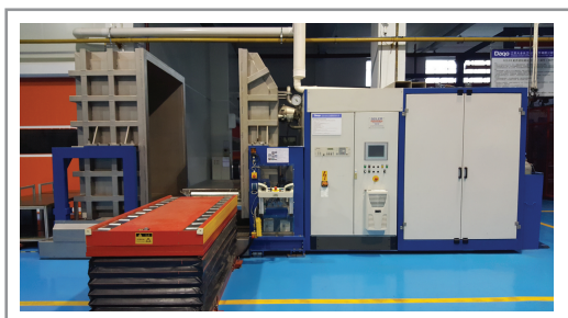
SEILER 公司的全自动氦检设备 Automatic helium leak detection equipment
